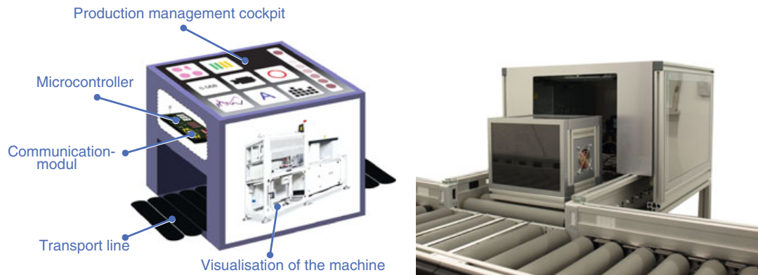
Fig. 1 Machine tool demonstrator—schema and original
